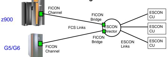
Exploit FICON Channel with Existing ESCON Control Units
